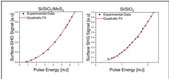
**Fig. 1**. Intensity of the surface-SHG signal vs pulse energy for different surfaces to verify a second harmonic signal.
